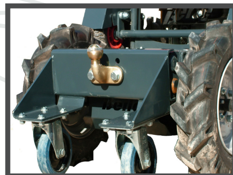
TOWING-EYE ATTACHMENT CAPABLE OF PULLING 1000KG
